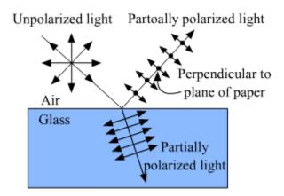
When unpolarized light falls on a refracting medium some part of the light is refracted and some part is reflected. These reflected and refracted light is partially polarized and separated by an angle of  $\pi/2$ . The reflected polarized light is called polarisation by scattering.
