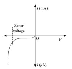
A Zener diode is fabricated by heavily doping both *p* and *n* sides of the junction. Because of the heavy doping, a very thin (<10<sup>-6</sup>*m*) depletion region is formed between *p* and *n* sides. Hence the electric of the junction is extremely high (~5 × 10<sup>6</sup> v/m)
