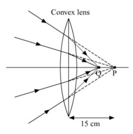
Here the object is a vertical object at *P*. According to sign convention, Object distance = u = +15 cm Focal length = f = +10 cm
