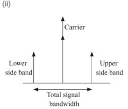
**Side Bands:-** Side bands are produced by modulations. The signal produced after modulation consist of frequencies slightly higher and slightly lower than the frequency of carrier wave (fc + fm and fc - fm) called sidebands.
