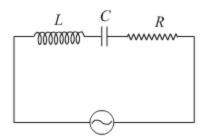
We get maximum current when the LCR Series Circuit is at resonance.
