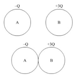
After the contact charge will redistribute equally on both the balls, the new charges on both conducting balls are:
