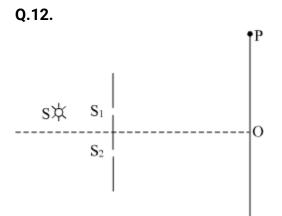
The figure shows a modified Young's double slit experimental set-up. Here SS<sub>2</sub> – SS<sub>1</sub> =  $\lambda/4$ .
