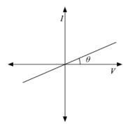
When an external resistance is also connected in an electrolyte, the voltage across the electrodes will reduce, so does the current in the circuit. If we plot a graph between Current in the circuit and the voltage, it still is a straight line but with the lesser slope. The slope of the graph will reduce because of the presense of external resistance in the circuit. Which simply means for the same value of current the circuit with external resistance.
