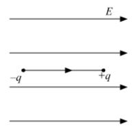
This is stable equilibrium because the potential energy of the dipole here is minimum. As,
