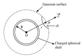
Suppose, we have to calculate the electric field at the point *P* at a distance r (r > R) from its center. A Gaussian surface is drawn through point P to enclose the charged spherical shell. The Gaussian surface is a spherical shell of radius r and center *O*.
