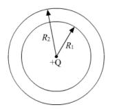
Because of the induction, the inner surface will occupy a negative change '-Q' and the outer surface will occupy a positive charge '+Q'.
